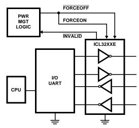
FIGURE 4. CONNECTIONS FOR MANUAL POWERDOWN
