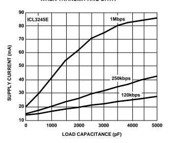
FIGURE 19. SUPPLY CURRENT VS LOAD CAPACITANCE WHEN TRANSMITTING DATA
