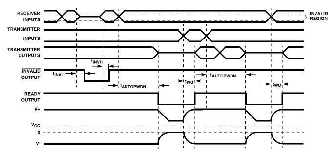
FIGURE 9. ENHANCED AUTOMATIC POWERDOWN, INVALID AND READY TIMING DIAGRAMS
