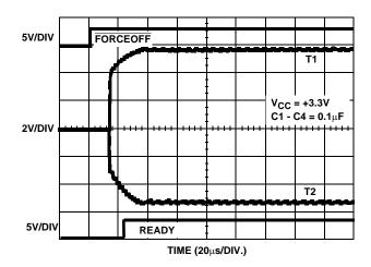
FIGURE 10. TRANSMITTER OUTPUTS WHEN EXITING POWERDOWN
