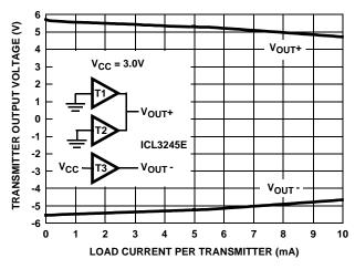
FIGURE 11. TRANSMITTER OUTPUT VOLTAGE vs LOAD
