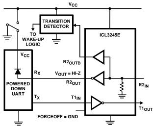
FIGURE 3. DISABLED RECEIVERS PREVENT POWER DRAIN
