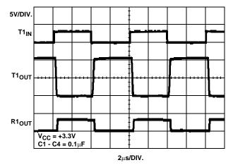
FIGURE 13. LOOPBACK TEST AT 250kbps (CL = 1000pF)
