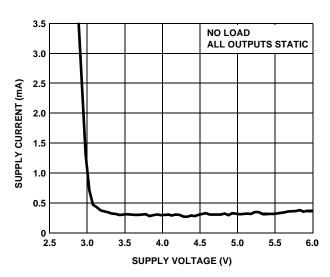
FIGURE 20. SUPPLY CURRENT vs SUPPLY VOLTAGE
